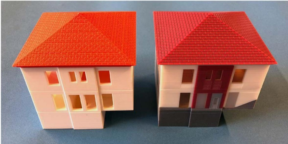
Figure 4. Printed models: FDM (left), PolyJet modelling (right)
