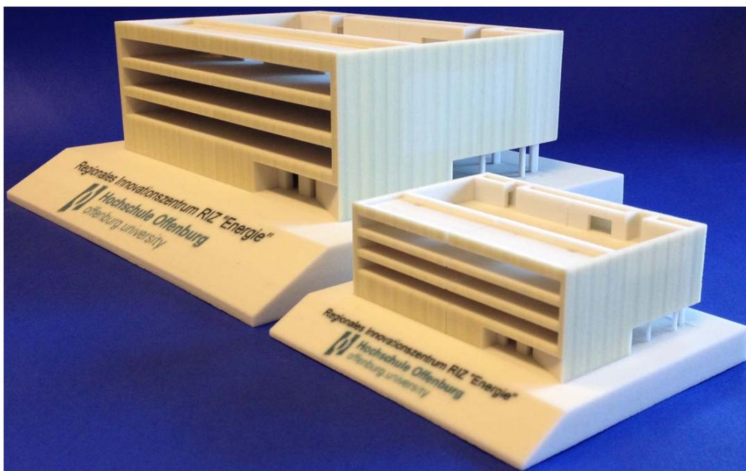
Figure 6. Parametrized architectural model in scale 1:250 (left) and scale 1:500 (right) manufactured by Binder Jetting
