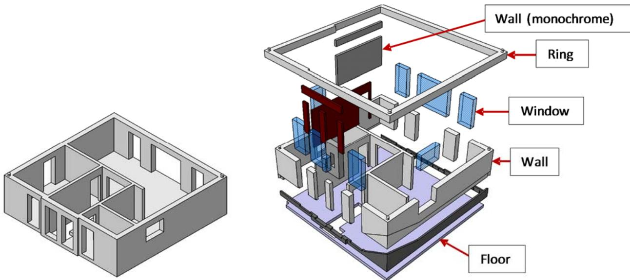
Figure 2. Separation of the ground floor (left) original volume, (right) Redesign with separated and coloured sub-volumes (exploded view)
