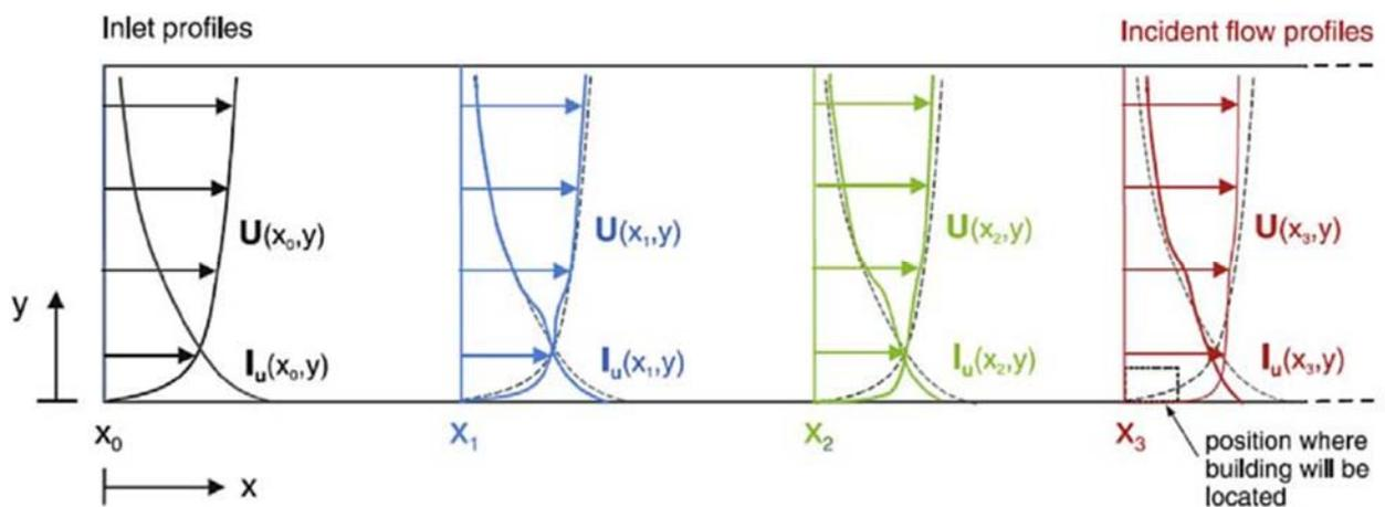
Figure 2. Schematic illustration of the development of an internal boundary layer (horizontal in-homogeneity) in a CFD simulation in an empty domain [72]
