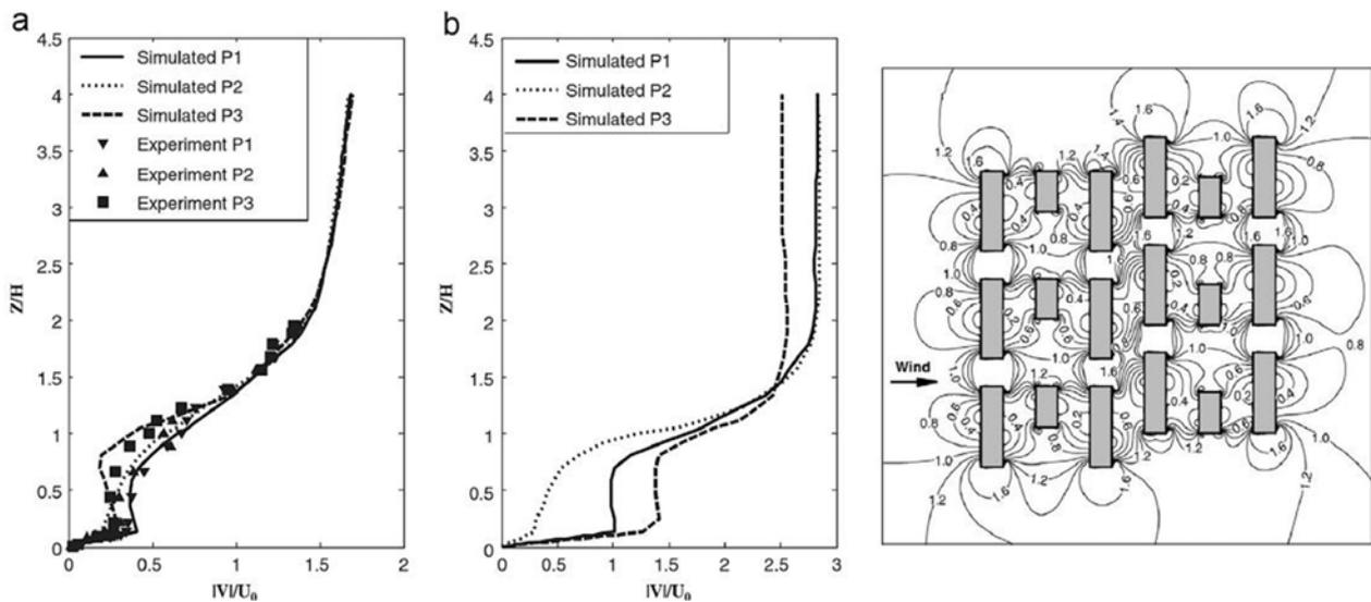
Figure 4. Experimental and numerical normalized wind velocity: (a) S–N wind and (b) computed normalized velocity field at 2 m from the ground level for S–N wind direction [94]
