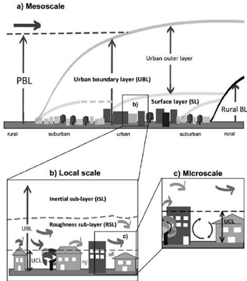
Figure 1. Sketch of urban boundary-layer structure indicating the various sub-layers and their names [72]
