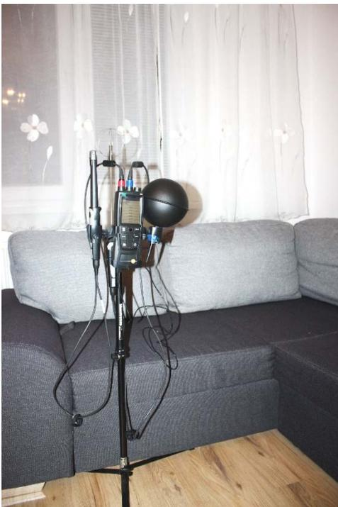
Figure 6. Measurement 1,1 m above the floor level in standpoint A
