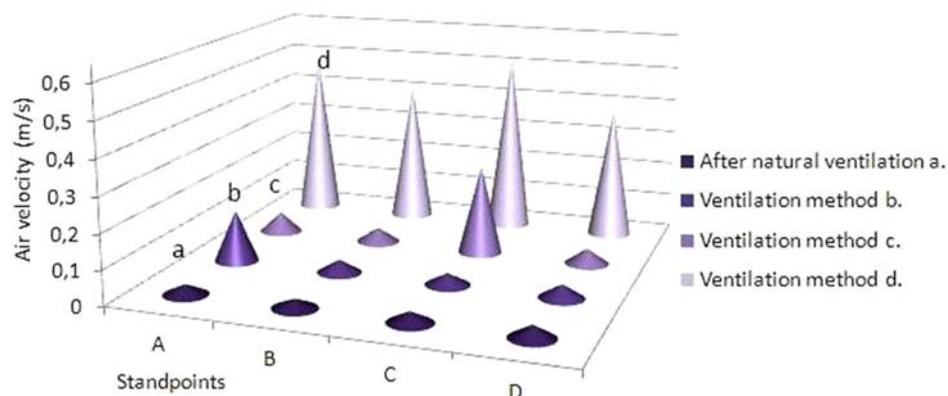
Figure 13. Values of air velocity in the height level 1,65 m
