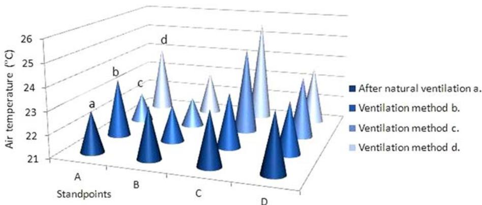
Figure 11. Values of air temperature in the height level 1,65 m
