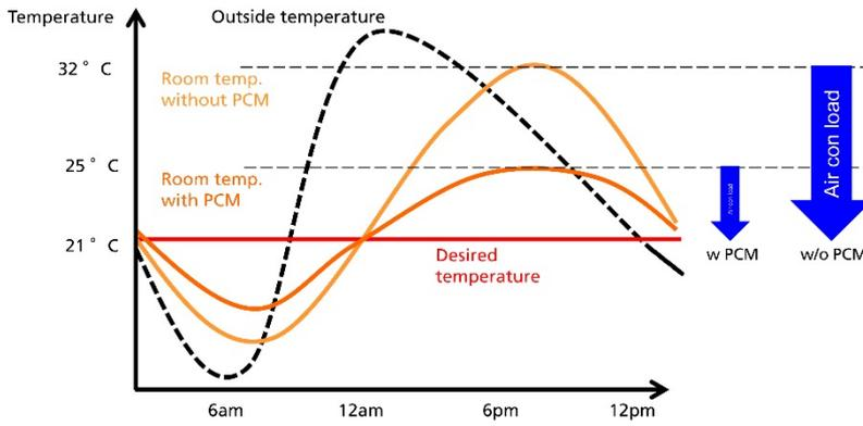
Graph 2. Temperature oscillations with and without PCM glazing Components (with PCM glazing components reduce necessary cooling power) [6]
