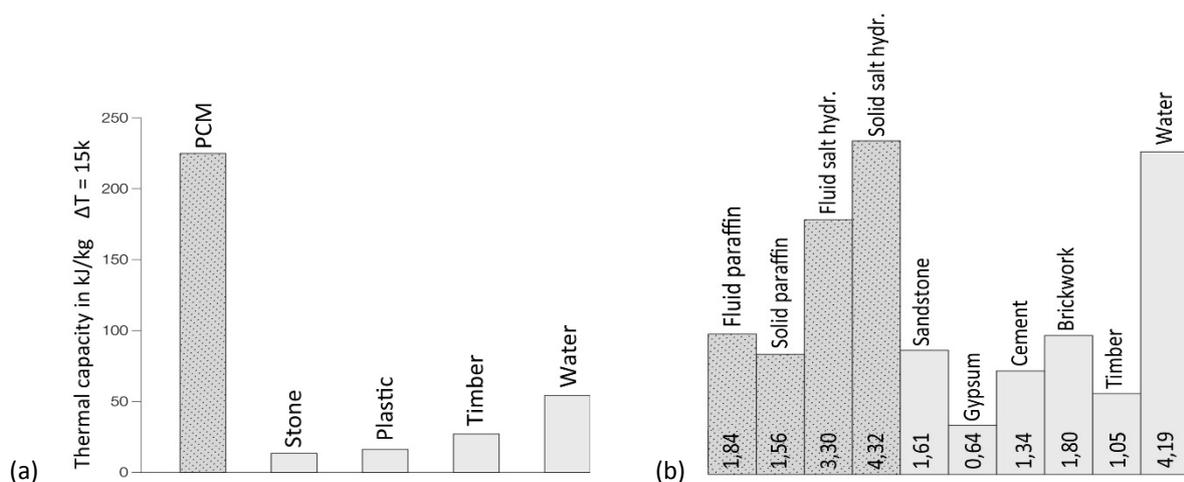
Graph 1. (a) Increased storage capacity through melting enthalpy [5] (b) Perceptible thermal storage capacity (kJ/L°C) for 1 litre, [5]
