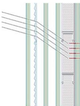
In winter, when the angle of incidence is lower than 35°, the reflective layer integrated in the first package of the thermopane does not reflect the sun rays.
