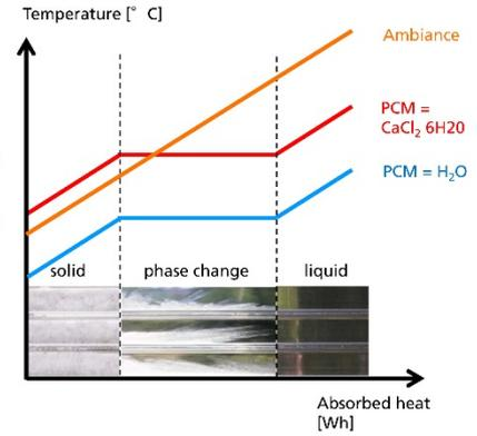
Graph 3: PCM-integrated (potassium-chloride-hexahydrate) glazing systems [6]
