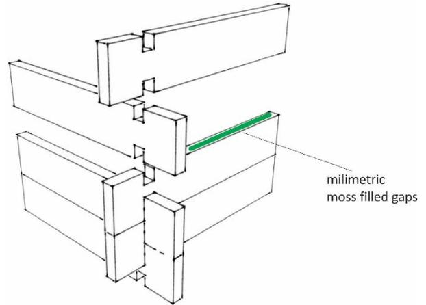
Figure 5. Middle zone construction and fitting of elements
